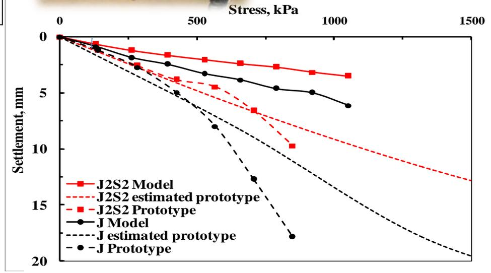
Settlement ~ Failure stress (field & lab. tests)
