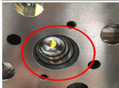
Dent on Injector Bore
